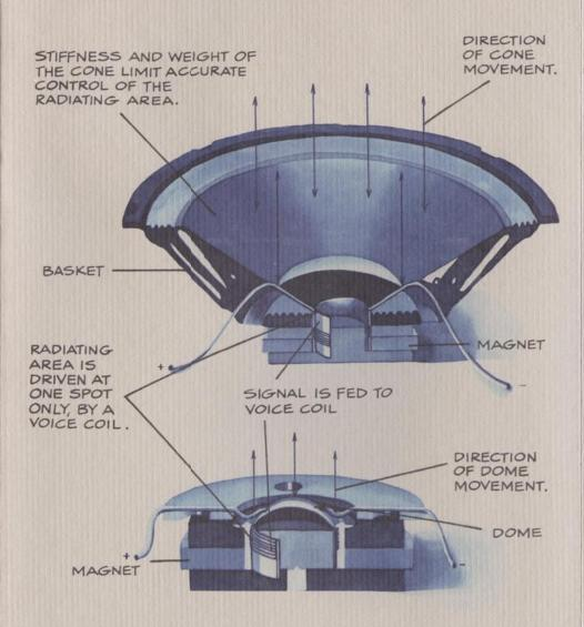
The response of cone and dome tweeters to transients, or sudden peaks in the music is inherently limited by their technology. This limited ability to accurately follow rapidly-changing input signals results in a "veiled" sound, lacking clarity, transparency and delicacy. The problem is most noticeable at high frequencies; cymbals, bells, guitar and violins lack their true life-like timbre.
