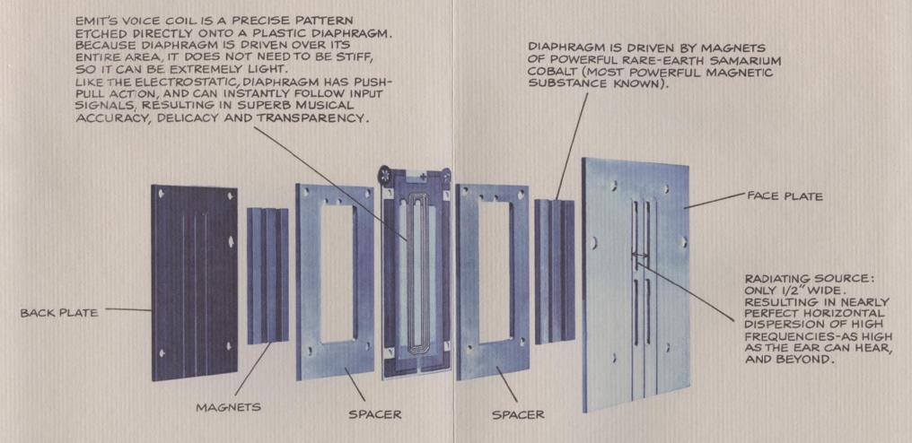
This is a view of the component parts of Infinity's Electromagnetic Induction Tweeter (EMIT). It is the magnetic analogue of the electrostatic; it achieves its drive from powerful magnets rather than from high voltage.
